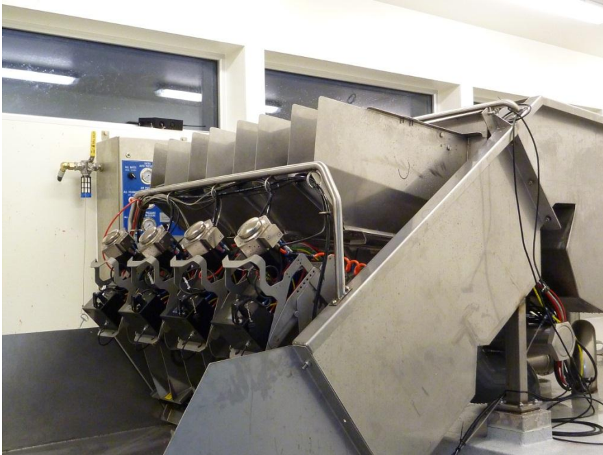
4 channel SI-7 combos mounted on a combination module, raised in cleaning position.
